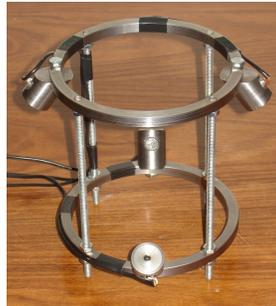
Figure 3: 3D Anemometer.
